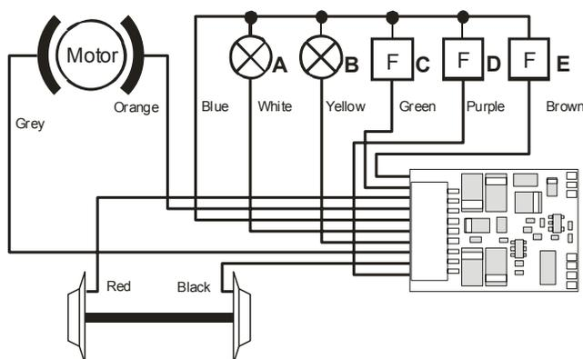
If the bulbs for the directional headlights are floating (isolated against wheel pick up and chassis) and connected according to above figure, they will shine brighter compared to using the rail as a common and the directional headlights will function while operating on conventional DC layouts.
